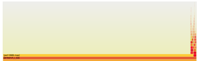
Figure 8: Perf [18], along with Flame Graphs [22], aided the profiling of the Taint Rabbit. The figure illustrates a recording of the Taint Rabbit on perlbench. Most of the flames are caused by basic block instrumentation. Meanwhile, the flat area represents execution in the DBI's code cache. Its dominance is a positive result as time is not heavily spent on instrumentation (only 2% in this recording). Unfortunately, symbols required for generating the flames are not available as this code is JIT'ed. However, profiling helped discover a bottleneck related to shadow memory during development.
