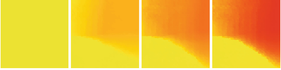
Fig. 1. Heat-map representation of executed rounds with time. Each device is depicted as a point located on its actual coordinates, time progresses from left to right. Devices start (left) with no round executed (yellow) and, with the simulation progression (left to right), execute rounds, changing their color to red. Devices closer to the static source (on the bottom left of the scenario) execute fewer rounds than those closer to the moving source, hence saving resources. (Color figure online)
